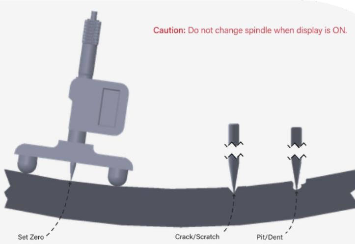
RajMet Digital Micrometer Depth Gauge is used to measure the depths of scratches, pits, dents and other surface defects on flat as well as curved surfaces, in materials such as Carbon Steel, Stainless Steel, Non-Ferrous metals, Plastic, Rubber & Composites.
